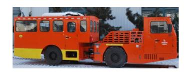
Superior stability and simple handling can improve the safety of underground lifts. The hydro brakes are more suitable for the complicated and difficult working environment of the underground to ensure safety. The cabin is framed to ensure stability, and all walking surfaces are non-slip to minimize the possibility of slips and falls.
