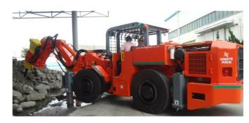
Higher productivity and efficiency is achieved by better stability and larger hammer size. The improved working mechanics of the rock breaker makes it easier to be positioned and stabilized.
