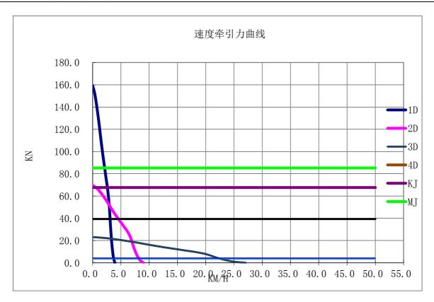
1D, 2D, 3D, 4D: Gear Positions; KJ is the static friction force at empty load, and MJ is the static friction force at full load; DK is the dynamic friction force at empty load, and DM is the dynamic friction force at full load;
