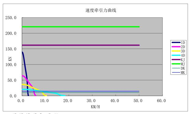
1D, 2D, 3D, 4D: Gear Positions; KJ is the static friction force at empty load, and MJ is the static friction force at full load; DK is the dynamic friction force at empty load, and DM is the dynamic friction force at full load;
