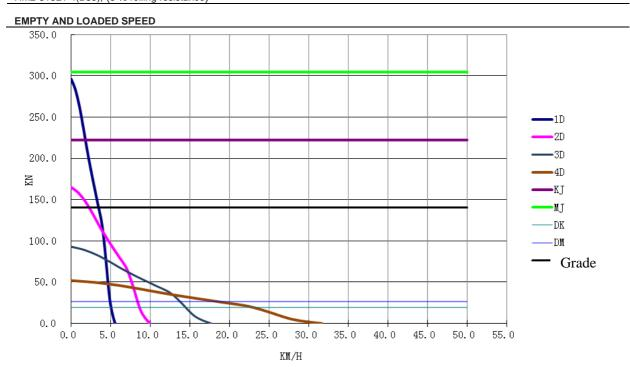
1D, 2D, 3D, 4D: Gear Positions; KJ is the static friction force at empty, and MJ is the static friction force at full load; DK is the dynamic friction force at empty, and DM is the dynamic friction force at full load;
